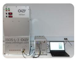
Photographs showing the typical setup of an ISOS-L-3 experiment. (1) First the device is mounted inside the ISOS-L-3 chamber and then the top plate is added. (2) The ISOS-L-3 chamber is carefully inserted into the test compartment of the ISOSun and water is added. You then switch on the solar simulator and run the preinstalled software.
